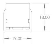
Flexible mounting profile Top or Side Bend or 3D 500mm
