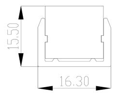
Flush Clip (note if using quick cap, end cap needs to be allowed for: 15.5mm x 15.5mm)
