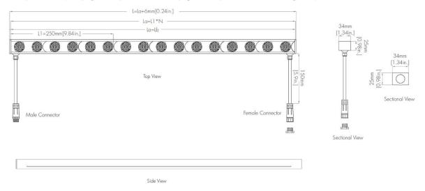
Power entry on the bottom (male plug at the input side and female plug at the output side as standard configuration)
